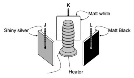
The student switched the heater on for 10 minutes. The thermometers were read before the heater was switched on. The thermometers were read again just after the heaters were switched off.
